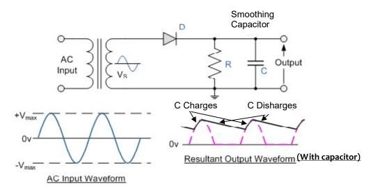
Fig.2: Half-wave rectifier circuit with capacitor filter
