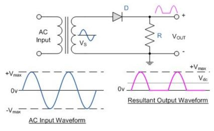
Fig.1: Half-wave rectifier circuit
